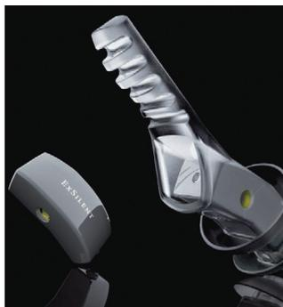
Helmbrechts also moulds the polycarbonate housing, mounted within the TPE tip itself, enclosing the battery, flexible circuitry, receiver, chip and microphone. The 14mm long, 7mm high PC housing represented a challenge in mould filling. This was resolved at Helmbrechts by flow path optimisation with use of flow aids and air vents.
