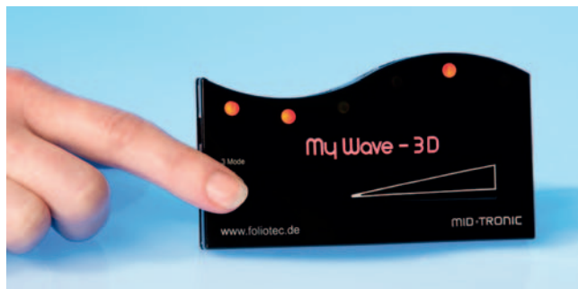
Fig. 4. The system displays the room temperature in binary form. The LEDs behind the numbers 1, 2 and 16 produce 19°C
