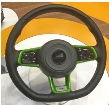
Steering wheel developed for GE-T with integrated switch and control functions, shown by Kunststoff Helmbrechts at K 2019
