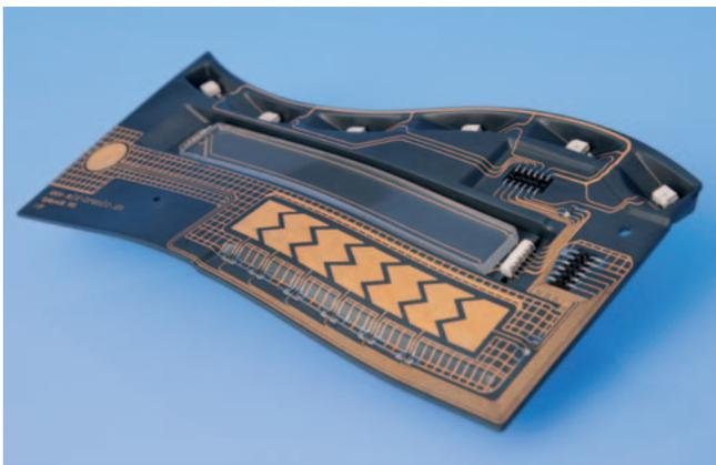
**Fig. 2.** The novel 3-D circuit board is provided with conductor tracks, capacitive surface (jagged region on the circuit board) and shielding (surrounding mesh surface)
